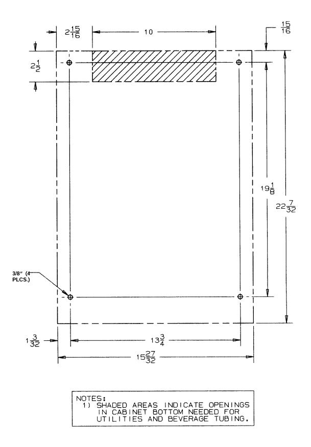
FIGURE 6. MOUNTING TEMPLATE DB90-BCZ
