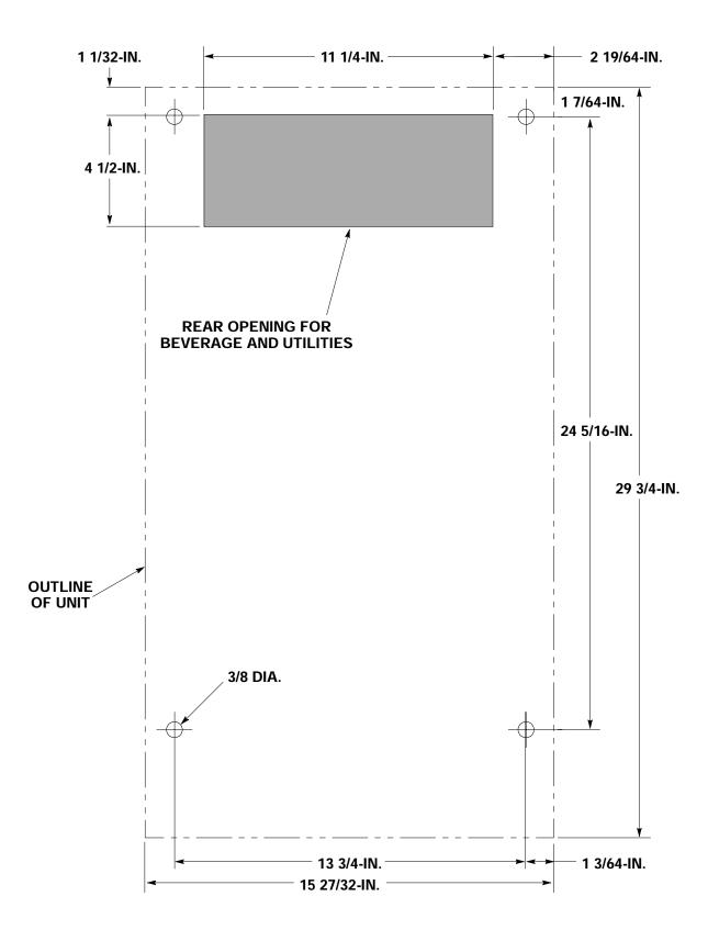
NOTE: 1) Shaded areas indicate openings in cabinet bottom needed for utilities and beverage tubing.
